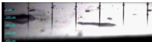
**Figure 6.** Drop formation of the water based ink with DMP-2831 printer.
